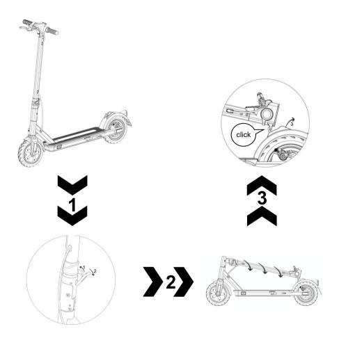
Make sure that your comscoot eco is switched off. To fold it, unlock the folding mechanism (first 1, then 2) and bend the handlebar stem. Then snap it into place on the rear mudguard. To open, pull the tab (3) on the rear hooking device on the mudguard. Now you can set up the handlebars and lock the folding mechanism.
