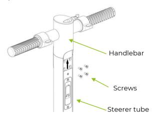
**OCAUTION:** The supplied spanner is only for pre-assembly. The screws must be tightened to the specified torque using a torque spanner.
