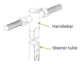
2. Secure the handlebar with the supplied bolts using a torque spanner. The tightening torque for the screws is 5 NM.
